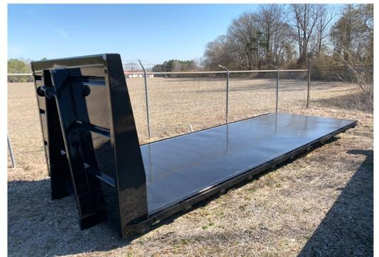
All Godwin hookloader bodies are manufactured using minimum ASTM mill certified grade 50 steel or greater. Godwin bodies are also zinc primed and powder coated tough for the highest standard corrosion protection in the industry.
